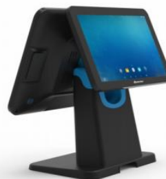
Dual screen • Main screen 15.6" sub screen 11.6" • IC/ID/NFC/MSR card reader
